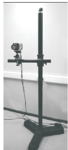
Figure 1. Shows variable offset in four calibrated IR cameras and camera mount.
